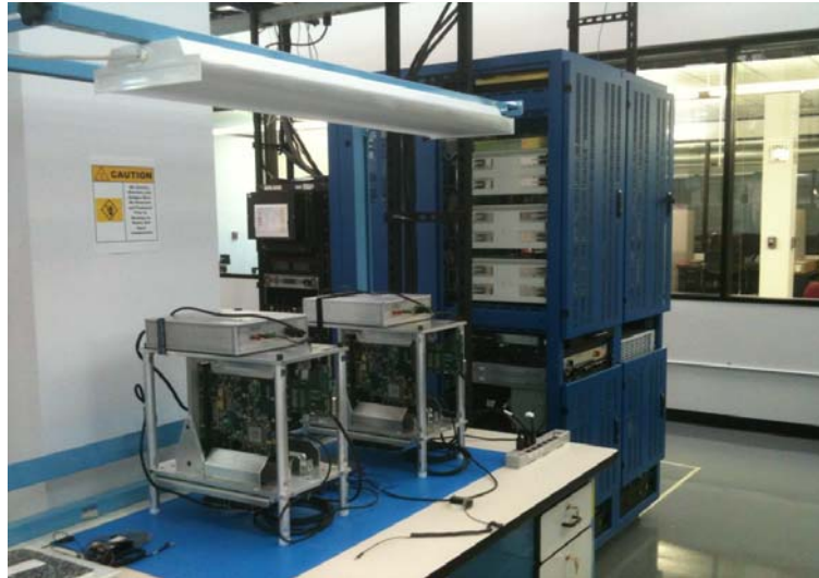
Kedalion built Test Bed with Honeywell Orion Flight Computer Brass Boards
