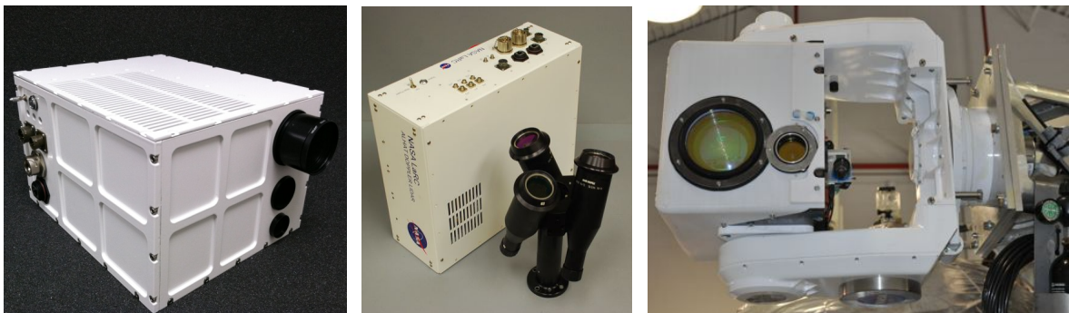
Figure 2. Stand-alone images of the ALHAT sensors: long-range Laser Altimeter (left), Navigation Doppler Lidar optics head and electronics box (center), and Hazard Detection System gimbaled flash lidar (right).
