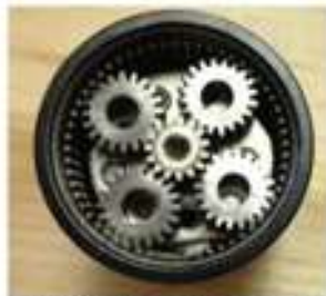
Gearbox with amorphous metal gears
