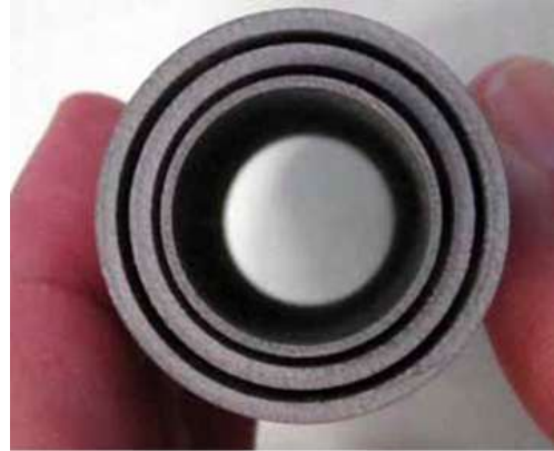
GSFC reentrant tube made by additive manufacturing for a cryogenic thermal switch for the ASTRO-H Adiabatic Demagnetization Refrigerator.
