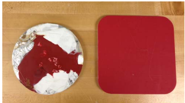
Figure 7. Example of HMC generation 1 tile (left) and planned generation 2 tile shape to improve storage and use for radiation shielding.
