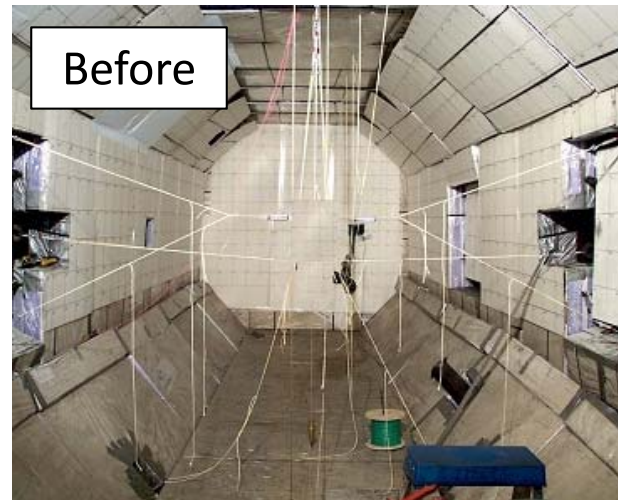
Examples of the before (without target) and after impact views of the target chamber (10 ft × 20 ft).
