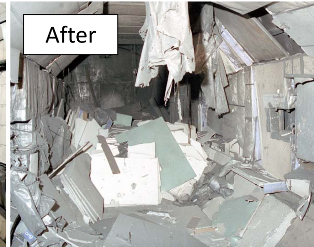
Examples of the before (without target) and after impact views of the target chamber (10 ft × 20 ft).
