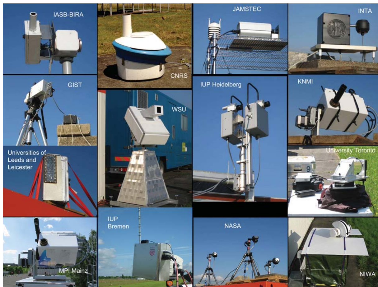
Fig. 3. Snapshots of the various optical instruments installed at the remote sensing site indicating the large variety of optical detection system designs actively involved in the campaign effort. Some images display complete stand-alone systems (e.g. WSU), others are only displaying the telescopes (e.g. NASA) that are connected to the spectrographs and detection systems by optical quartz fibres.
