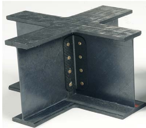
Figure 11. Photograph of a cruciform section test specimen.
