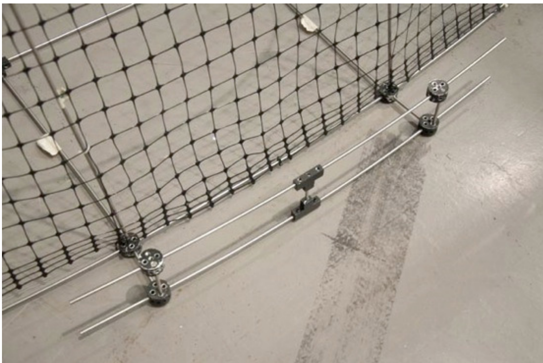
B-4. Phase 2 Mockup Details: Toe-kick/Simulated Platform Edge with Steel Rod and Connectors
