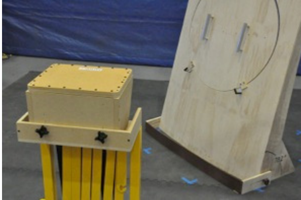
B-3. Phase 1 Mockup Details: GSE Shelf, Adjustable toe-kick, Handles on Clear Door
