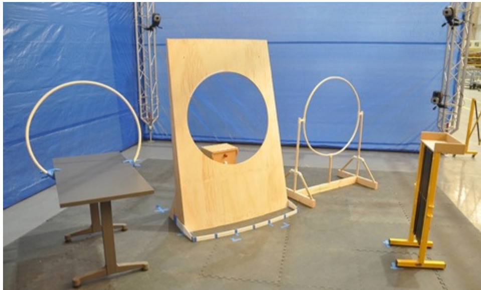
Figure 6.6-4. Vehicle Hatches, GSE Shelf and Platform, Battery LRU Mockups used during Phase 1
