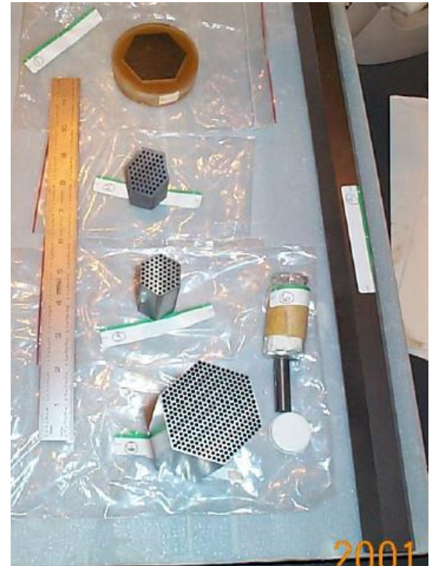
W-UO 2 CERMET Samples fabricated during ANL Program
