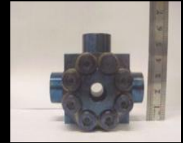
FM Cell (Transmission View) (500 bars/600°C)
