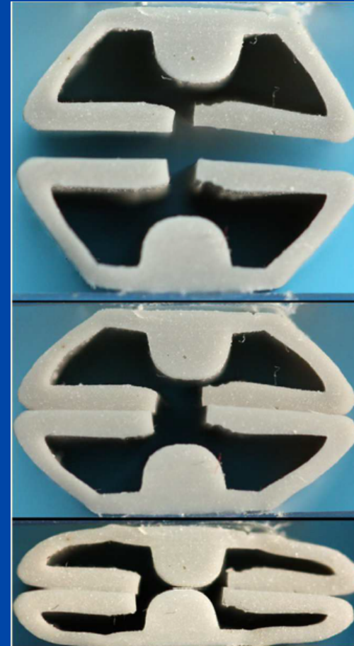
Seals with retractable “shrouds”
