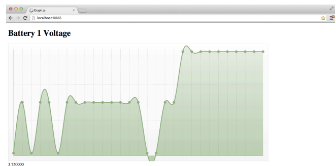
Figure 3. Entire set of rover data: 4 min 3 sec test - Battery 1 Voltage
