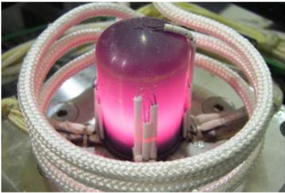
Figure 1.—Thermal standard test article: Type-K thermocouples were welded on this specimen, which was used for furnace development and temperature testing.
