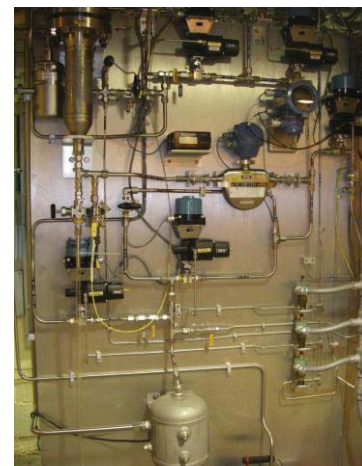
Figure 15: Green Propellant Flow Panel
