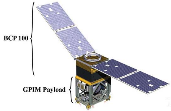
Figure 3: GPIM Payload on the BCP-100 Spacecraft BCP: Ball Configurable Platform
