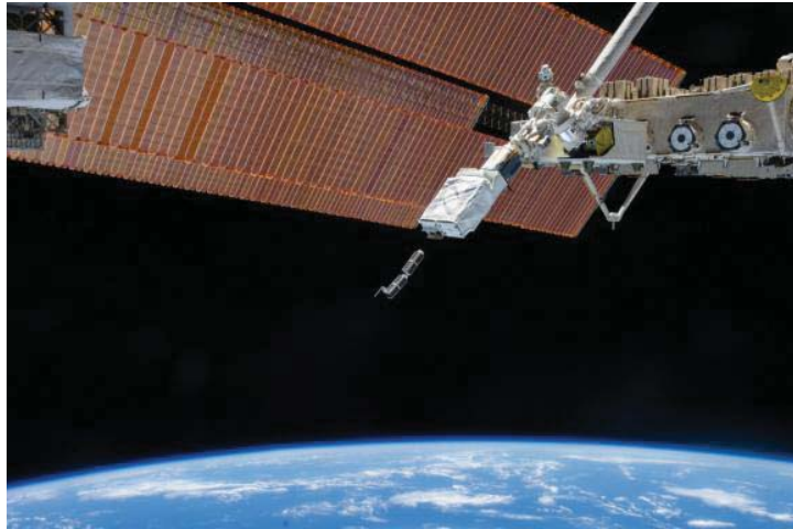
Figure 1: The Japanese Kibo robotic arm on the International Space Station deploying Planet-Labs CubeSats
