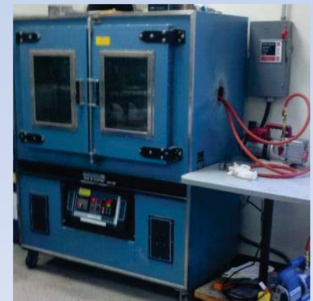
Oven Cure of Panel Under Vacuum
