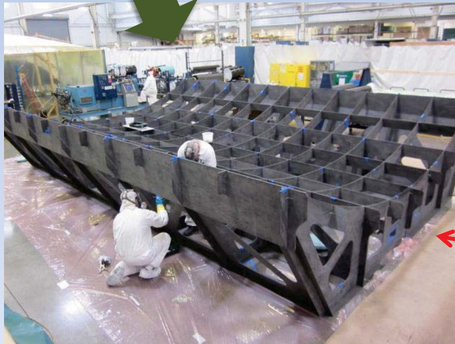
1/6 th Tool Fabrication
