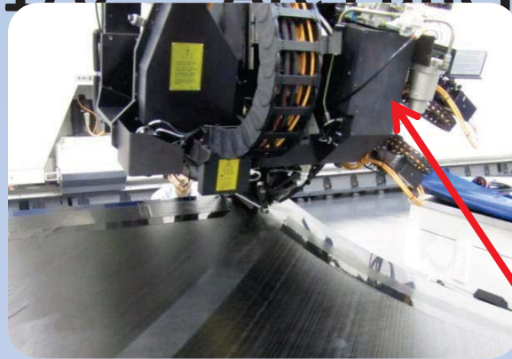
Automated Fiber Placement System
