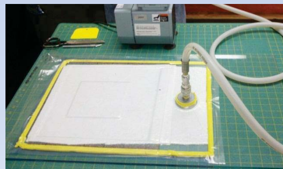
Vacuum Debulk of Composite Panel
