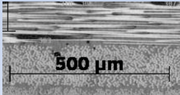
[0,90] Composite Microscopy Image
