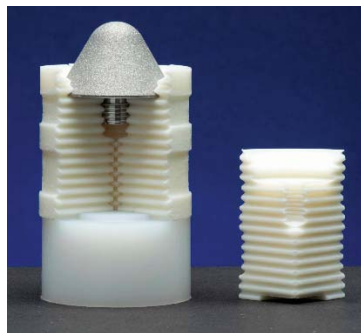
Fig. 3. Photo of launch package for open front sabot.
