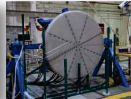
Heat shield Test Setup at Dryden
