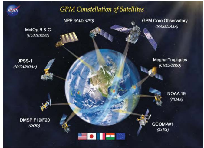
Figure 6: Illustration of the multiple precipitation measurement satellites which comprise the GPM constellation (Image credits: NASA)
