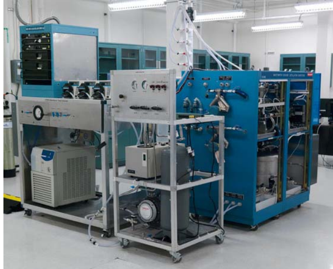
Figure 1. The CDS test system in the JSC AES Water Lab. The Cascade Distillation Subsystem (CDS) is contained in the blue box on right, and is supported by the AES Facility Support System contained in the silver racks on the left.
