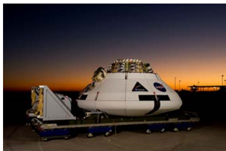
Figure 1. Orion CEV Capsule at YPG on its C17 Ejection Sled for Parachute Drop Testing
