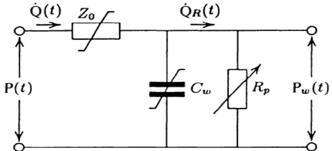
Three-element model used to compute aortic flow as proposed by Wesseling et al.  $Z_0$ , characteristic impedance of proximal aorta;  $C_w$ , windkessel compliance of arterial system;  $R_p$ , total systemic peripheral resistance;  $Q(t)$ , blood flow;  $P(t)$  arterial pressure waveform;  $P_w(t)$ , windkessel pressure
