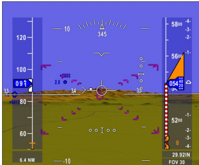
Figure 7a: Expanded view of SVS Display Concept PFD
