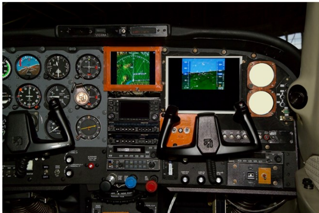
Figure 5: Synthetic Vision System Display Concept
