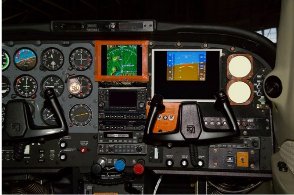
Figure 3: Single-Cue Flight Director Display Concept
