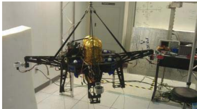
Extreme Access prototype during tethered flight testing.
