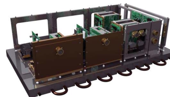
Cut away of NASA 300V PPU
