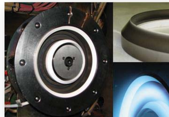
JPL H6 with magnetic shielding
