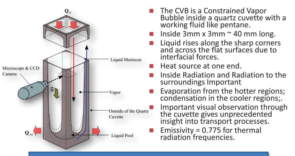
A transparent "heat pipe" – ideal for studying basic fluid flow and heat transfer due to interfacial forces inside.
