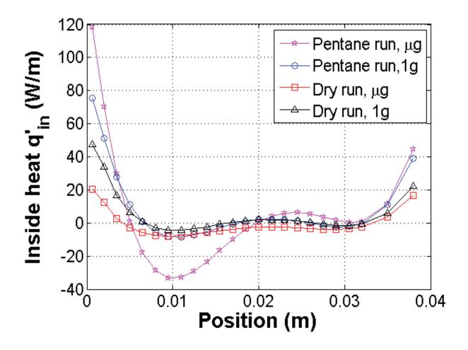
Inside heat transfer per unit length for 2 W in  $\mu g$ . Only radiation present on inside and outside for the dry case. Net inside radiation field is thereby known.
