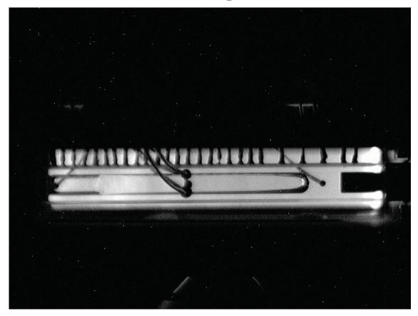
Visual Observations Support Experimental Heat Transfer Results Based on the Temperature Profile Note: Excess fluid at hot end.
