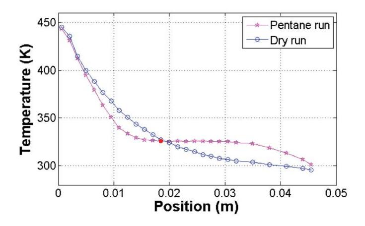
TEMPERATURE GIVES OBVIOUS CHANGE IN AXIAL CONDUCTION GRADIENT PER UNIT LENGTH, EXTERNAL RADIATION AND INSIDE HEAT TRANSFER
