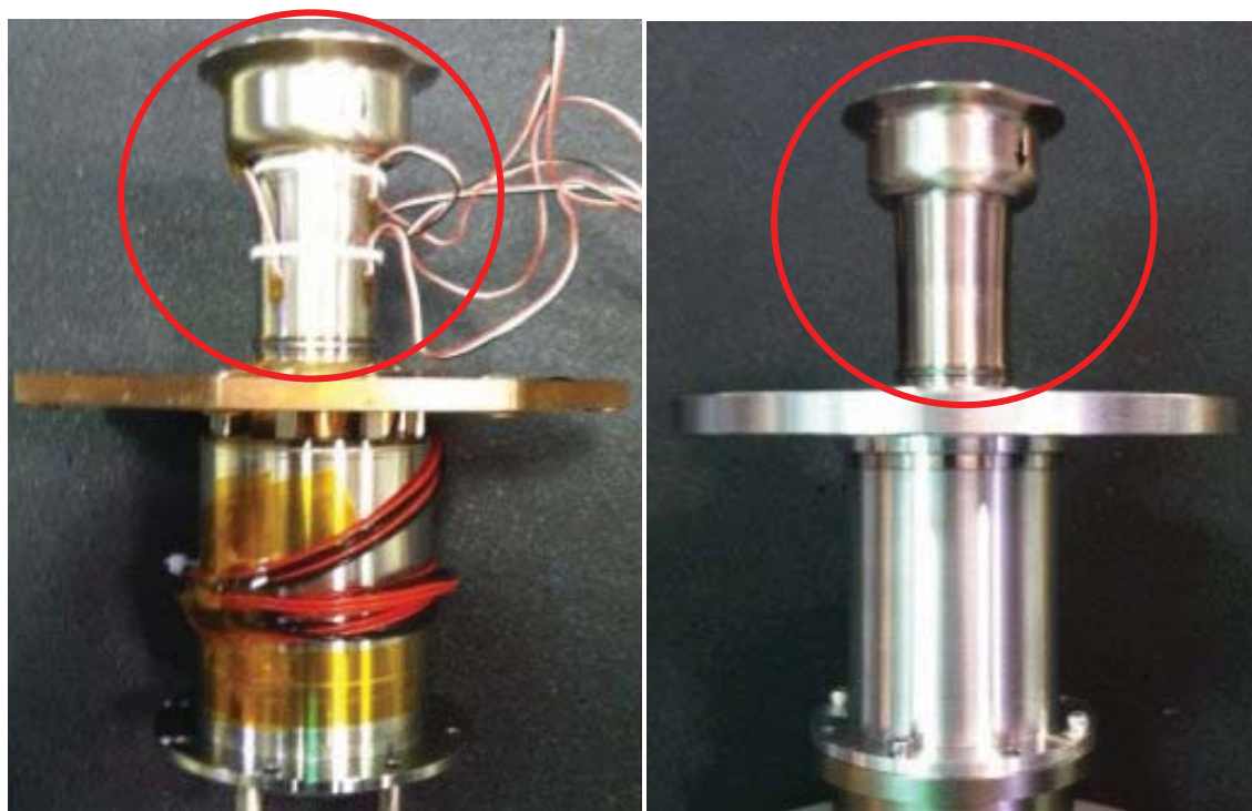
Figure 2.—Advanced Stirling Convertor (ASC) mockup with G05 (left) and ASC dynamic simulator with G02 (right). Heater heads are circled.
