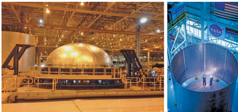
Fig. IX: SLS core stage confidence dome weld (left) and barrel section at MAF
