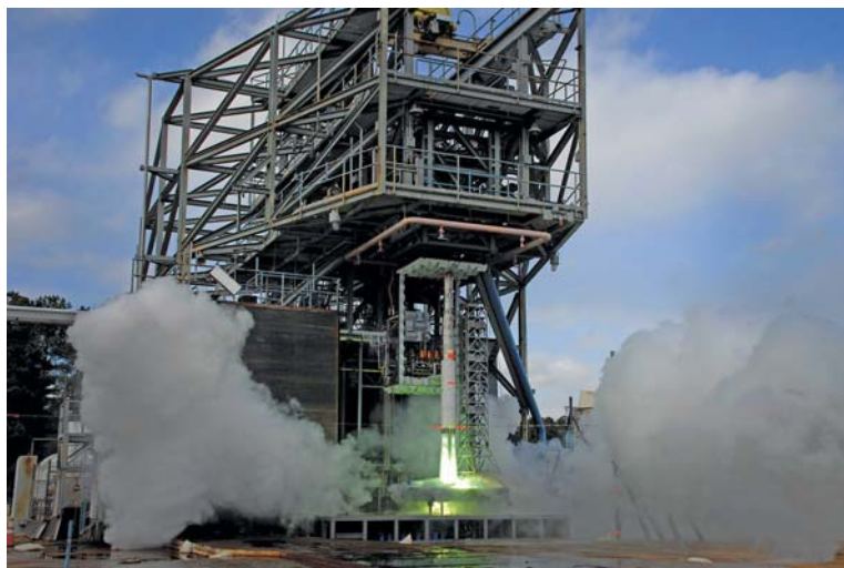
Fig. XIV: Core stage SMAT testing at MSFC
