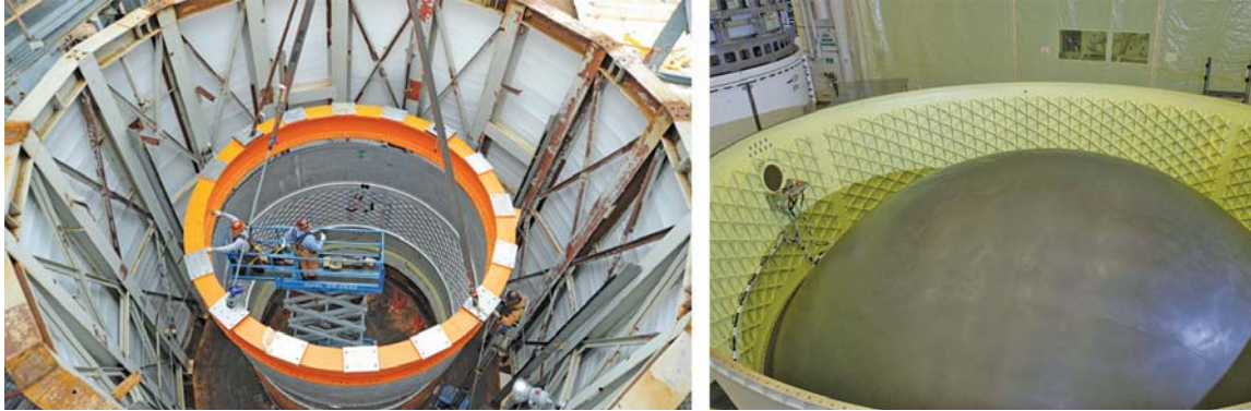
Fig. X: Orion stage adapter test article in stand (left) and flight stage adapter/diaphragm
