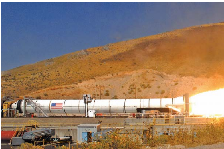
Fig. VII: SLS 5-segment Development Motor (DM-3) test firing
