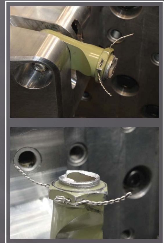
2 nd Development Test: Forward Lug Fatigue Failure
