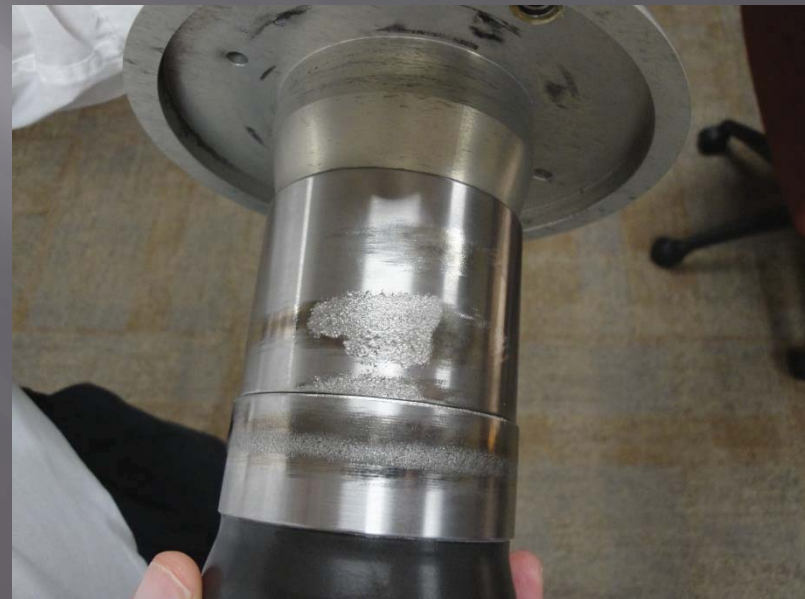
SAFJS Assembly Wear Post Vibration Testing
