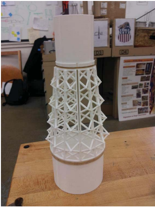
Figure 7. A scaled model of Brigham Young Universities isotruss interstage built out of ABS plastic.
