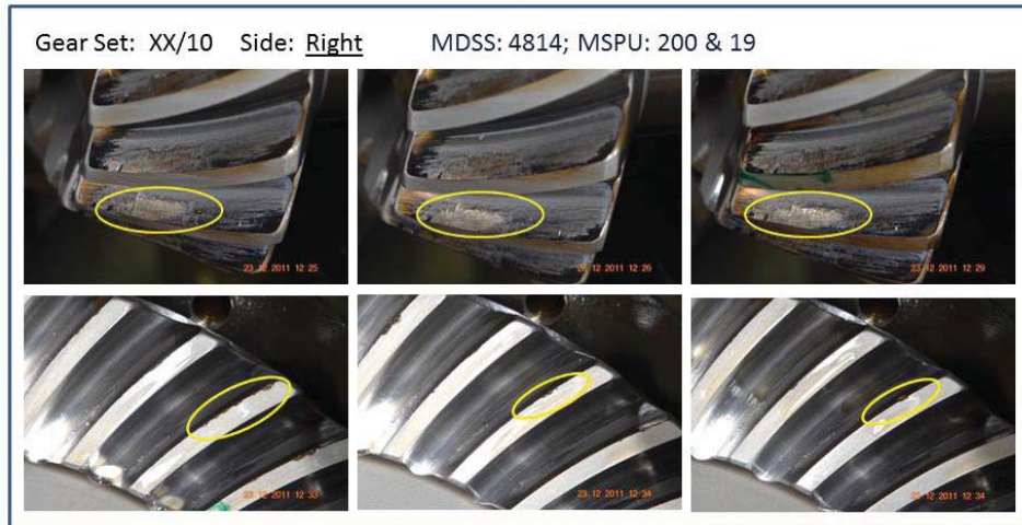
Figure A.1.2.—Test 1 gear and pinion damage modes.
