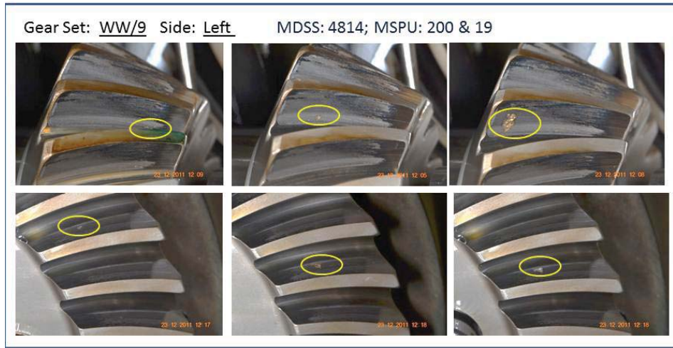
Figure A.1.1.—Test 1 gear and pinion damage modes.
