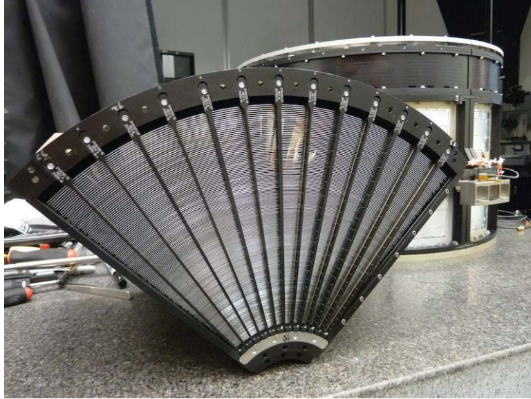
Fig. 3 ASTRO-H FM2 fully populated housing of 203 shells and the completed FM1 is in the background. There are 13 alignment/support bars, on each phase, each with 203 grooves that hold the 203 shells by the edges
