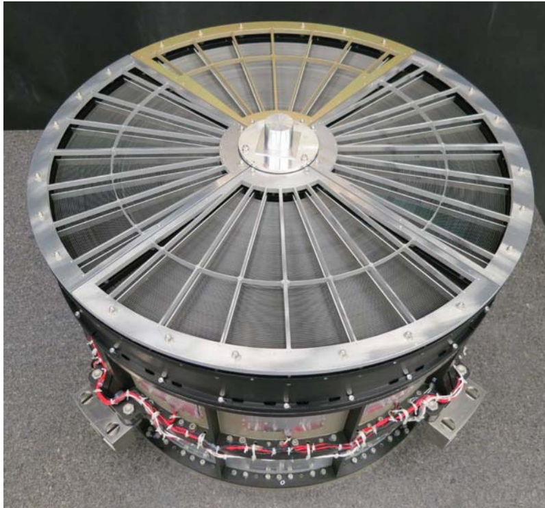
Fig. 6 ASTRO-H FM1 integrated mirror with corresponding pre-collimator (PC, from Nagoya University) on top of each quadrant, and one thermal shield frame(TS, from Nagoya University) on one of the quadrant
