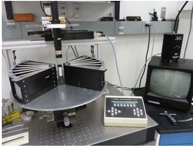
Fig. 4 Alignment setup in polar coordinates. Precision and repeatability of the translation stage was at 1\ \mu\text{m} , and wobble of the rotation axis was at 1\ \mu\text{rad}
