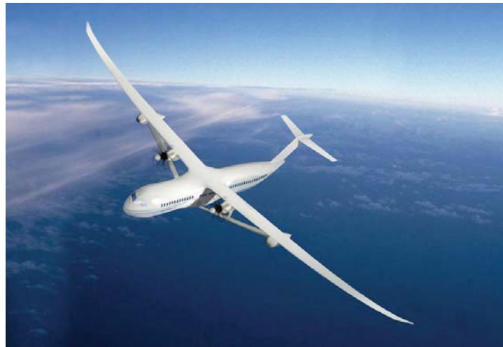
Figure 1. Boeing SUGAR Truss-Braced Wing (TBW) Aircraft Concept
