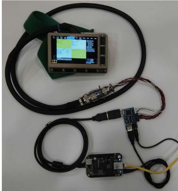
Figure 1: Beaglebone Black computer driving the Desert RATS cuff display
