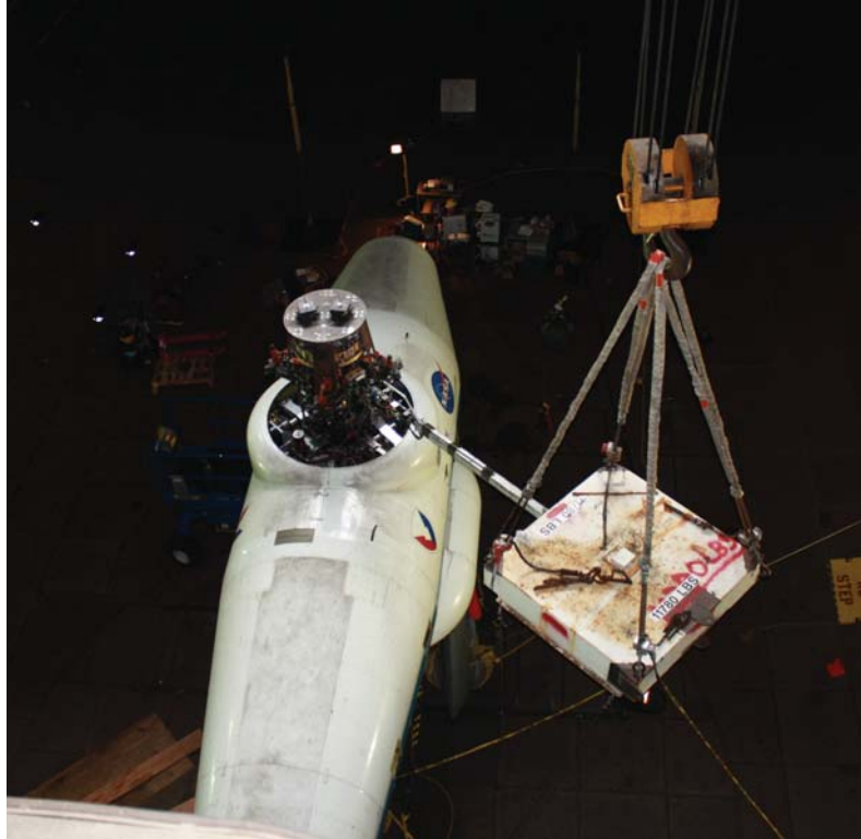
Figure 1. Shake test installation. In-plane shaking at 45° azimuth
