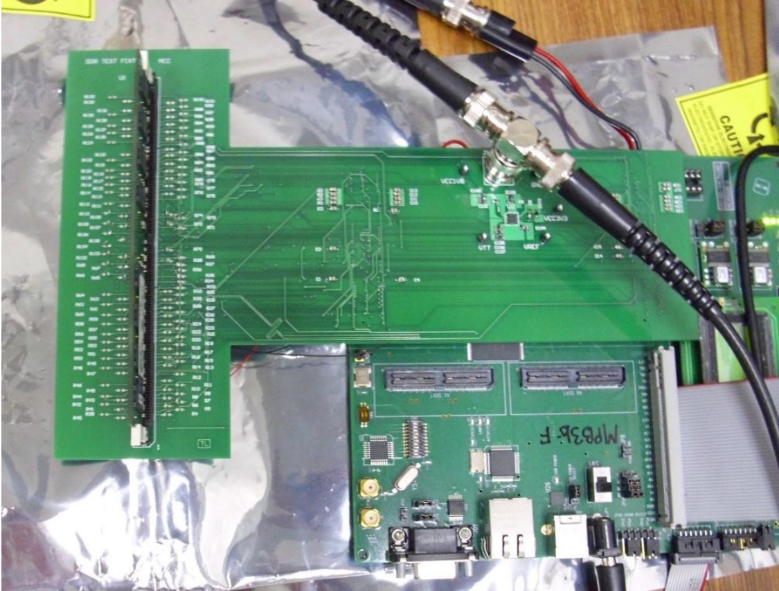
Figure 4.2-2. MPB3b-based test system as developed in FY12. This system was expanded to include multiple boards that will enable many devices to be tested simultaneously.
