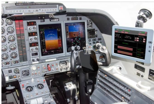
Figure 8. EFB installation in the Avanti Cockpit.
