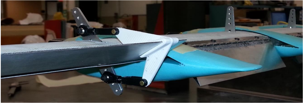
Figure 8. GL-10 Control Surface Double Link Actuation
