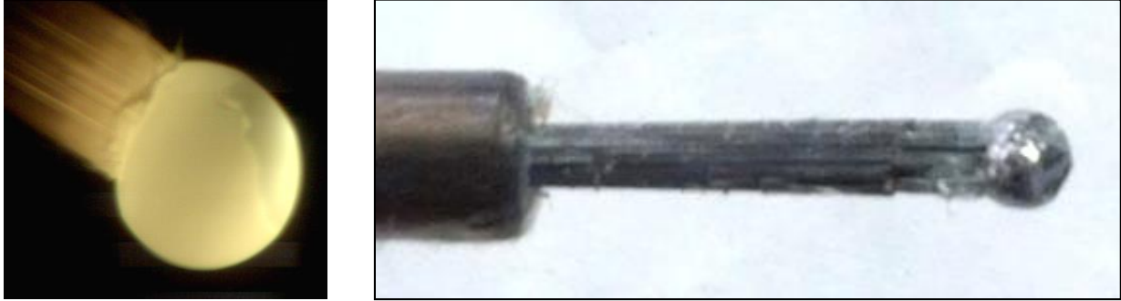
Figure 1. Boron ball attached to the boron fiber bundle. The bundle diameter is about 1/8 inch. (a) shows an image of the molten ball while it is being heated by a 5 kW CO 2 laser inside a BNNT production rig; (b) shows the boron ball at room temperature, after re-solidification.
