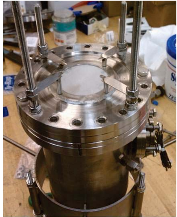
Figure 13.—Completed LAD Screen/Cup Assembly
