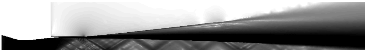
Figure 8. Density gradient view of Seiner nozzle, nozzle exit Mach number = 2.0, NPR = 7.82.
