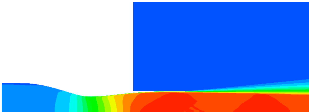
c) USM3D 2014 Mach profile with k-ε turbulence model with enhanced Sarker’s compressibility correction.
