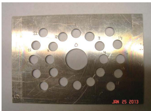
Figure 1.—Sample holder plate used in the 35 kHz hyperthermal asher.
