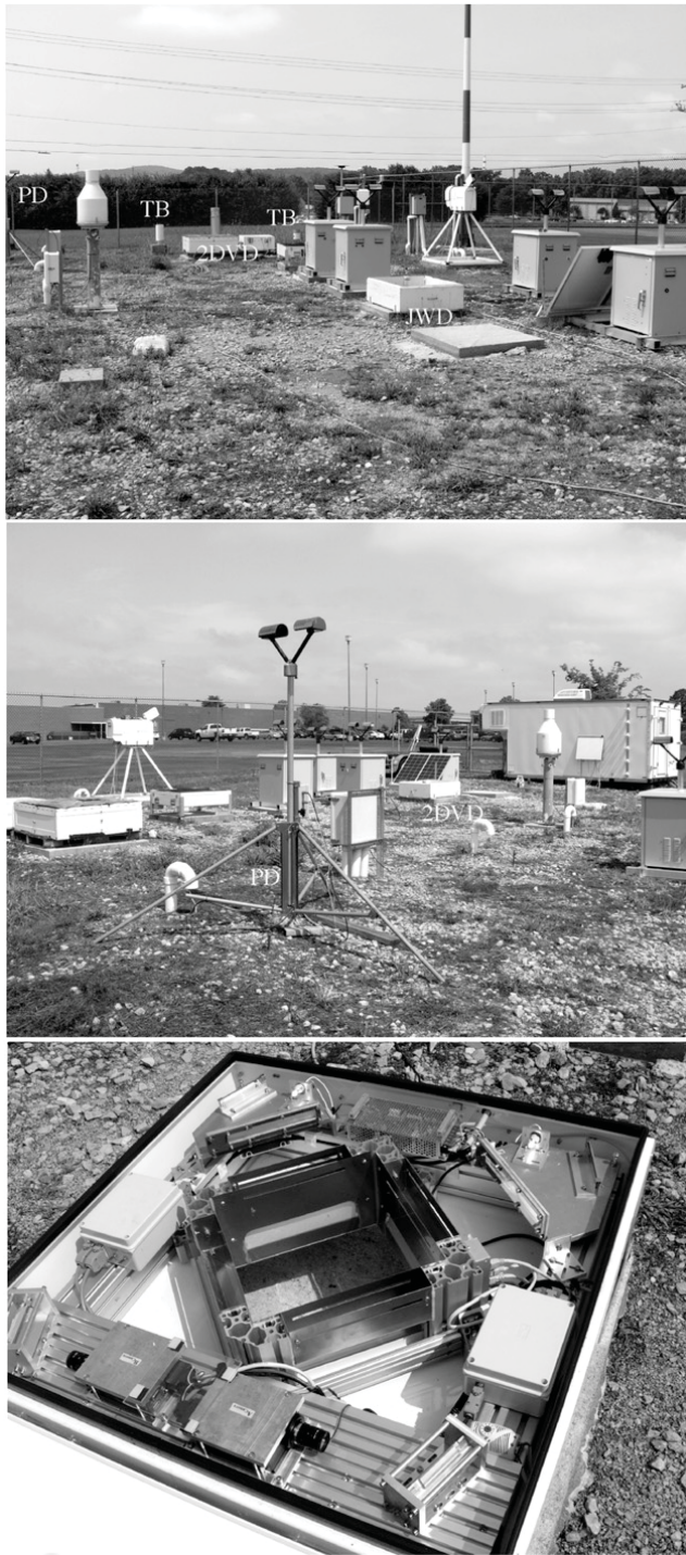
FIG. 1. In situ precipitation measuring test site. The instruments used in this study are labeled as (top) JWD sensor inside the white painted box, TB rain gauge back to the right and one of the secondary TB gauges back to the left; (top),(middle) 2DVD in the back, and PD on the left and in front, respectively. (bottom) A close look at the third generation of 2DVD.
