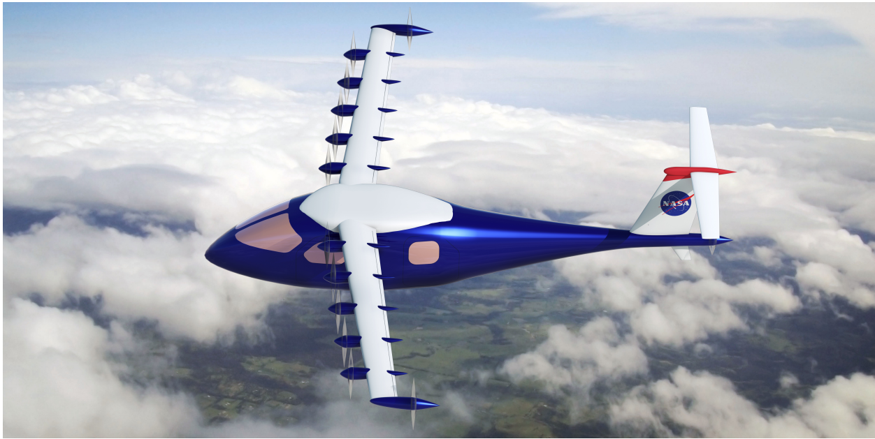
Figure 1. An early conceptualization of the LEAPTech aircraft, with ten leading edge-mounted propellers.
