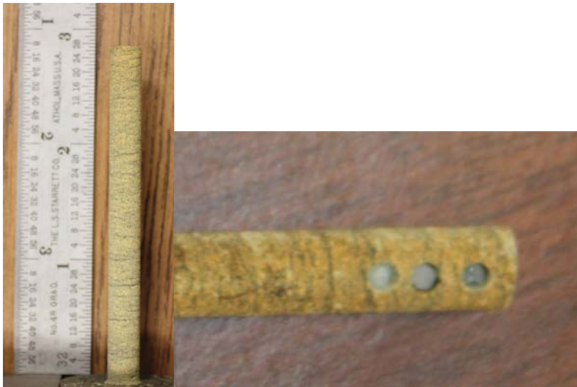
(a) (b) Figure 3: (a) PICA cylindrical test coupons (6.35mm diameter) (b) seeded materials inserted in the PICA prior to encapsulating
