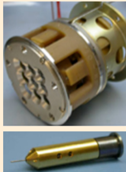
Figure 2: Busek CMNT thruster head and single emitter (9 emitters per thruster head).
