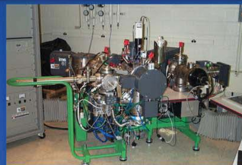
Secondary Ion Mass Spectroscopy (SIMS, Cameca IMS-6f): It uses secondary ions from sample surfaces to identify and quantify elements and their isotopes. It is sensitive to all elements and impurities at ppm levels. Can map locations of all elements including hydrogen, incorporate elemental distribution, depth profile, and quantitative analysis. Requires flat polished samples and very high vacuum.
