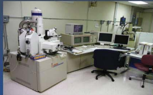
JEOL Superprobe(JXA-8900R): Scanning Microprobe allows for precise chemical analysis down to ppm levels using x-rays. Uses four spectrometers with a large chamber size that can accommodate either fractured or flat samples.
