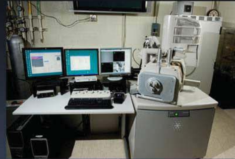
Field Emission-SEM (FEI Quanta 600): Provides very high resolution and depth of field. It can examine metallic, non-metallic, and wet samples up to 12 inches in diameter. Uses EBSD to evaluate grain orientations. Resolution is 2nm@30KV, magnification range is 7x to 1Mx. In pressure under 20 Torr (maximum), with particle analysis systems and SSD energy dispersive spectrometry (EDS).
