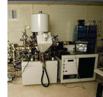
Kratos AXIS Ultra: Instrument uses both white and monochromatic x-rays for depth analysis of thin surface films, including depth profiling. Can identify elemental compositions and oxidation states. Applications include coatings, polymers, and polymers.
