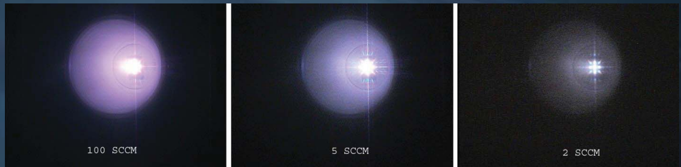
Inductively-coupled discharge (35-50 W) ~600-900 MHz
