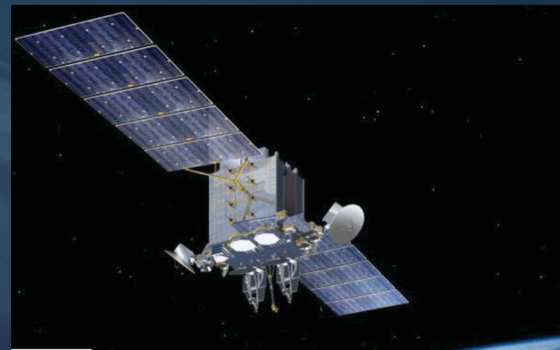
USAF AEHF – BPT-4000 Hall thruster (x4) 2010 (Geo Orbit – boosted system when bi-prop motor failed)
