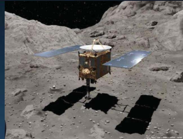
JAXA's Hayabusa – 10 \mu microwave ion thruster (x4) 2003-2010 (Itokawa – sample return)
