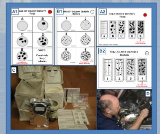
Microbial environmental sampling. Density charts are used during spaceflight to approximate the concentration of fungi (A) and bacteria (B) in the air (1) and surfaces (2). Specially designed flight hardware for air (C) and surface (D) sampling are used by crewmembers during flight.
