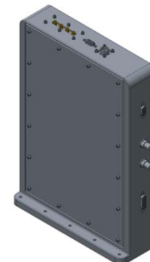
Interface Unit ( new ) Power conversion 1 PPS Time Signal Generation C&DH Formatting ISS Interface
